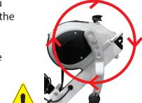
Winch handle Rotates Rapidly when unloading
