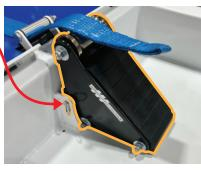
Retractable Gear Attachment in RGA Bracket
