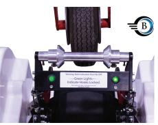
When on ice or other slippery surfaces unlock the cradle rotation. In the event that one tire looses traction the tug can start turning abruptly. This can cause damage to your Aircraft & Lazy Susan due to the twisting force it applies.
